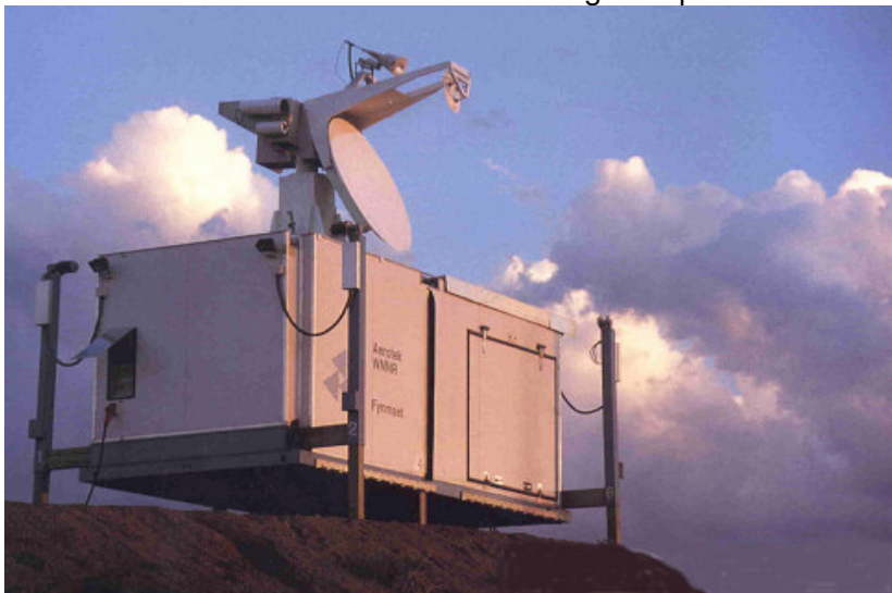
Figure 8 Fynmeet dynamic RCS measurement facility
