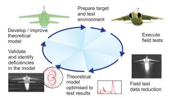
Fig. 7. The signature modelling and development cycle.
