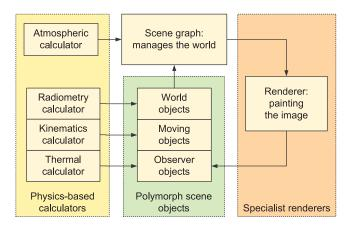
Fig. 8. Primary software functions in the simulation.
