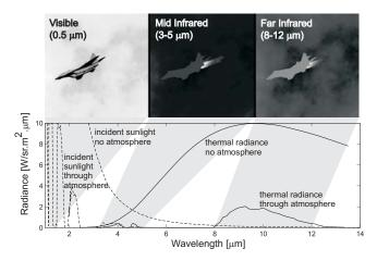
Fig. 3. Optical signature in several spectral bands: the solid line is self-emittance and the broken line is reflected sunlight. The target has 80% emissivity. The images show rendering of an object in three different bands.
