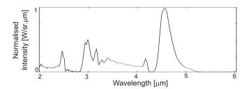
Fig. 4. Normalised spectral radiant intensity of a gaseous radiator.
