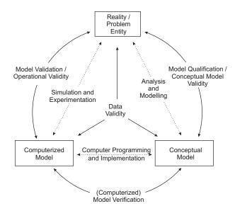
Fig. 9. Simplified Version of the Verification and Validation Process [5], [6].
