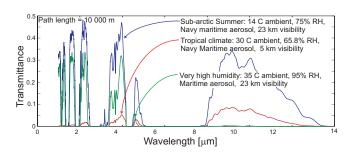
Fig. 6. Atmospheric transmittance at sea level, calculated with MODTRAN.
