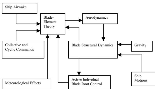
Fig. 1. Blade-sailing aeroservoelastic scheme
