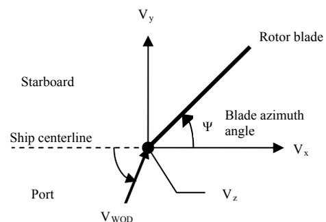
Fig. 4. Flow velocity components for the WOD conditions
