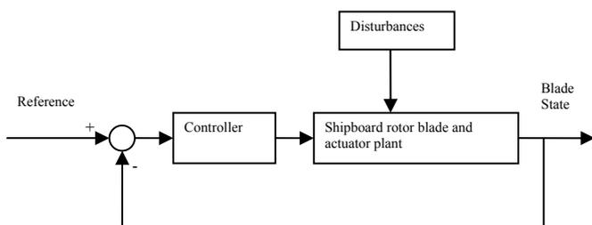
Fig. 2. Blade-sailing feedback control system
