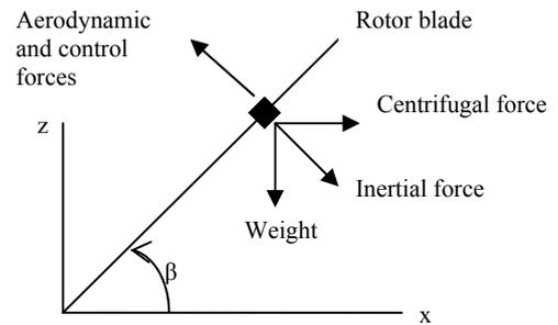
Fig. 3. Forces at a flapping planar blade-element for the proposed blade-sailing model (rotating frame)
