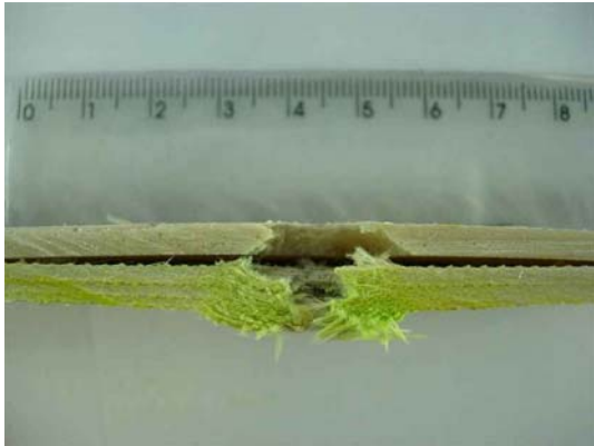
Fig. 3. 38 caliber impact in a P3 nanocomposite
