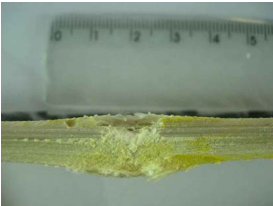
Fig.4 9 mm FMJ impact in a P2 nanocomposite
