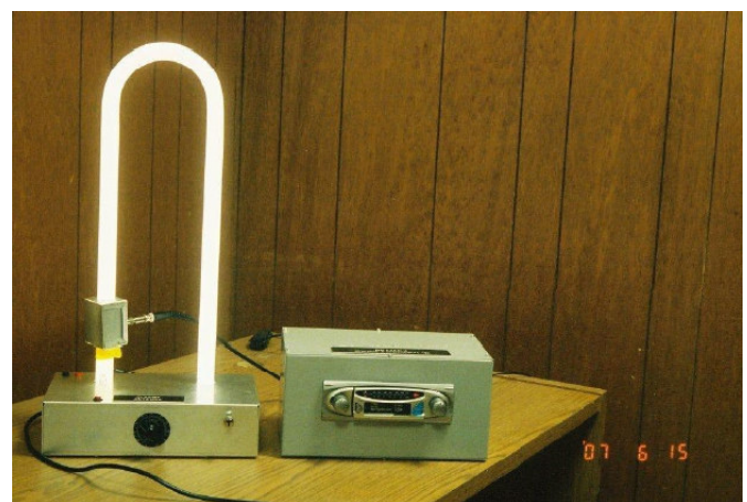
Fig. 4 – A plasma antenna connected to a radio [13].
