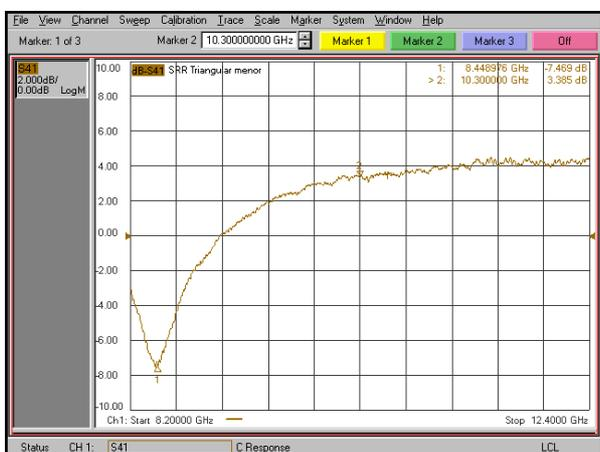
Fig. 7: Magnitude S41 para *bulk* Triangular (55 mm x 95 mm x 51 mm)
