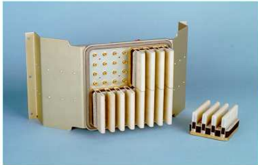
Fig. 8 - Modular sub-array radiating elements
