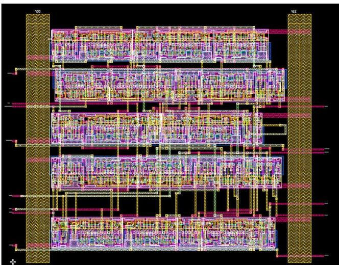
Fig. 6. Final layout of the Single-clock CLB
