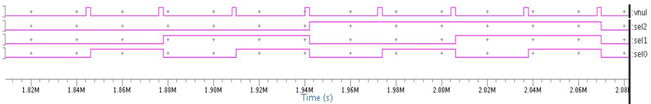
Fig. 5. Temporization signals for the sampling period of the Control Logic Block (CLB).
