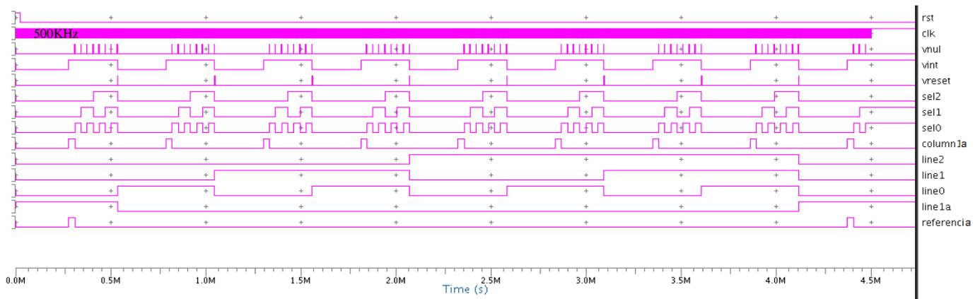
Fig. 4. Input and Output signals of the Control Logic Block (CLB).
