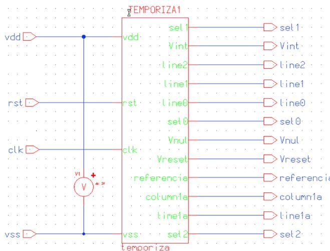
Fig. 3. Generated Test Bench through Design Architect, in IC Studio, by Mentor Graphics
