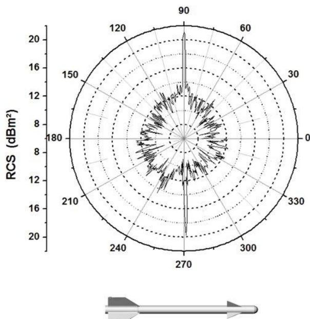
Fig. 7. Polar plot of the measured RCS of a missile. RCS units in dBm². The missile figure at the bottom shows the orientation of the missile. Radar frequency 10 GHz.
