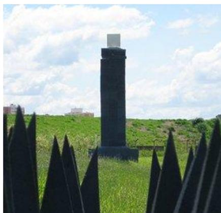
Fig. 3 Open range RCS facility. Support pylon for RCS measurements (background; height, 8 m). The pylon is covered with pyramidal carbon black radar absorber. Pyramidal carbon black radar absorbers on the surface (foreground). Atop the pylon is a 1 m<sup>2</sup> metal plate used for calibration of the system.
