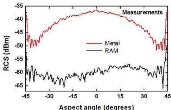
Fig. 5 RCS measurements of a 90° dihedral corner reflector. Radar frequency, 10 GHz. Metal surface and surface covered with a RAM. The aspect angle of 0° corresponds to the situation when the incidence of the radar wave is perpendicular to the vertex of the corner dihedral; at -45° and 45° the radar wave impinges perpendicularly on the surface of one the square plates.
