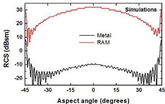
Fig. 6 RCS simulations of a 90° dihedral corner reflector. Radar frequency, 10 GHz. Metal surface and surface covered with a RAM. The aspect angle of 0° corresponds to the situation when the incidence of the radar wave is perpendicular to the vertex of the corner dihedral, at -45° and 45° the radar wave impinges perpendicularly on the surface of one the square plates
