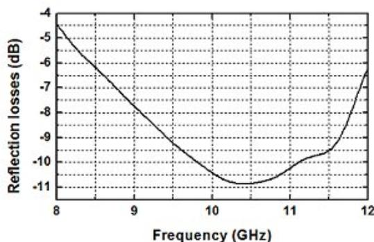
Fig. 4 Reflection losses as a function of the frequency. Iron carbonyl dispersed in a silicon rubber matrix. Thickness of the RAM is 2.5 mm.
