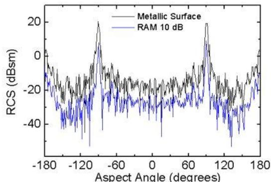
Fig. 8 Simulated RCS of an air-to-air missile. Metallic surface and surface coated with a RAM (attenuation, 10 db). Radar frequency 10 GHz.
