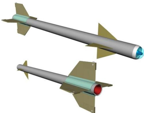
Fig. 1 Front and rear views of the CAD model of the air-to-air missile. Note the glass dome (light blue) protecting the heat-seeking device and the rocket nozzle cavity (red).
