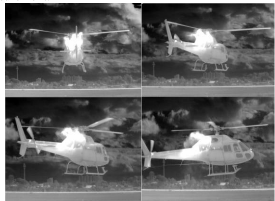
Fig.4 – H-55 during maneuvers in the hovering flight on ground effect during a turning from 6 to 3 hours aspect angle.
