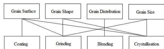
Fig. 1. Interdependency of Processes and Properties.
