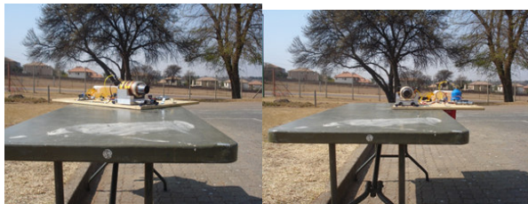
Fig. 4. View from the MWIR camera line of sight for aspect angles of 135^\circ (left side) and 180^\circ as used in AA scan session.
