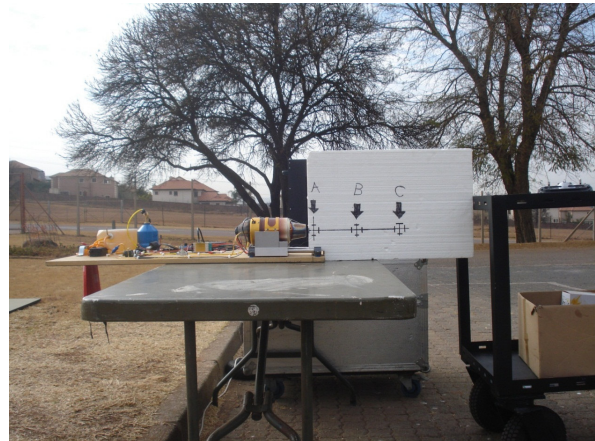
Fig. 7. Close-up of the mask used as reference to adjust the three FOV positions of the SR in the small FOV session.
