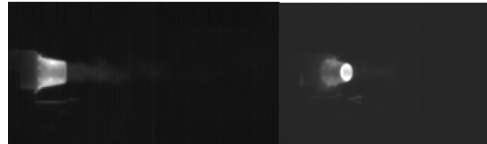
Fig. 12. Tail pipe recordings in the MWIR band for 90° (left) and at 135° aspect angles, both for 145k RPM. A 4% NDF filter was used in order to have no saturation in the tail pipe pixels.
