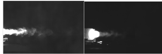
Fig. 11. Plume recording in the MWIR band for 90° (left) and for 135° aspect angles, both for 145 kRPM. No filter was used in order to have the plume radiance well above the detector noise level.
