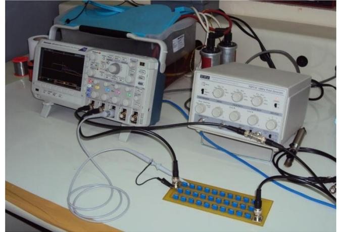
Fig. 3. Experimental set up for the NLTL tests.
