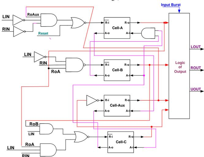
Fig. 10. Dme-fast-e: Net of control cells and logic of condition.
