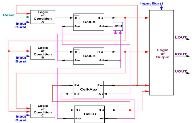
Fig. 9. Dme-fast-e: Net of control cells →connections (request and acknowledge).
