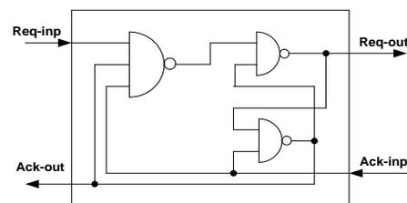
Fig. 1. Memory element: synthesis by direct mapping of [24].
