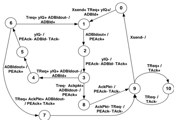
Fig. 5. BM Specification: HP-Pe-send-ifc controller
