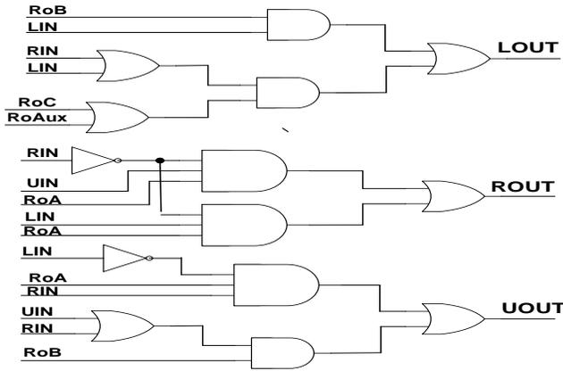
Fig. 11. Dme-fast-e: logic circuits of output signals.
