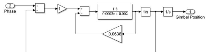
Fig. 5. Tracking loop.
