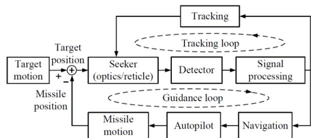
Fig. 1. Typical IR guided missile block diagram [4].
