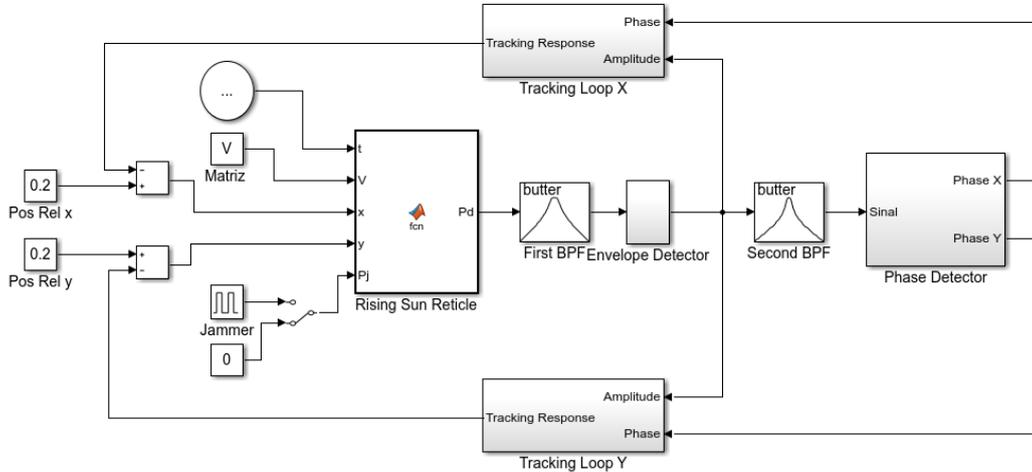
Fig.6 Simulation Model implemented in Simulink.
