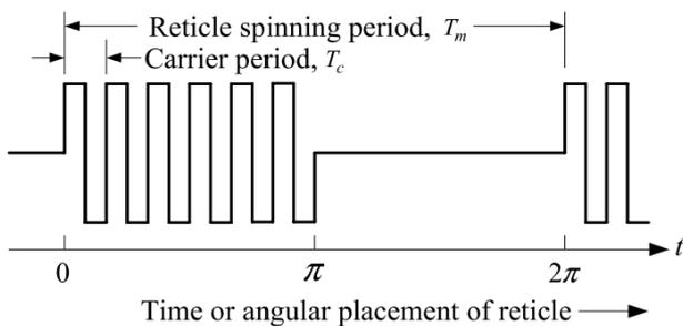
Fig. 3. Detector Output Signal [5].
