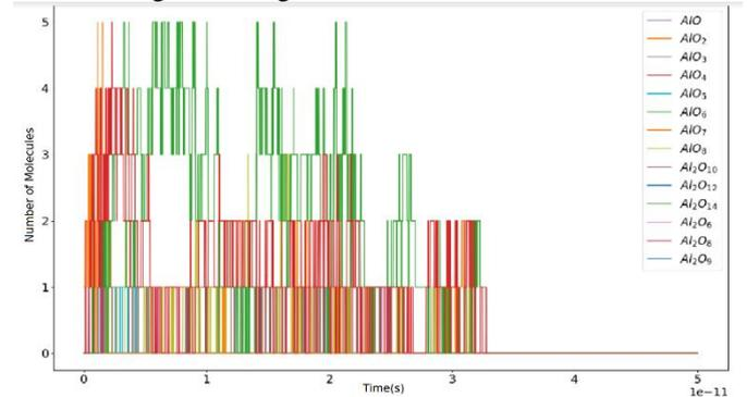
Fig. 3. Formation of Aluminum and Oxygen complexes during the combustion of the formulation with 1% (w/w) C and 5% (w/w) Al.
