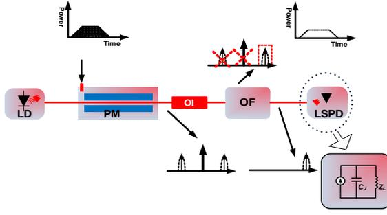
Fig. 1. Schematic diagram of the photonic ED. LD – Laser Diode, PM – Phase Modulator, OI – Optical Isolator, OF – Optical Filter, LSPD – Low-Speed Photodetector,  $C_j$  – Junction Capacitance, and  $Z_L$  - Output Load.
