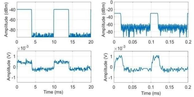
Fig. 5. The RF input signals power at 17 GHz are shown in the superior part of the figure. The pulse widths of the RF signals are 4 ms and 25  $\mu$ s from the left side respectively. The lower part of the figure show video signals voltage at 8 dB condition for TSS measuring.
