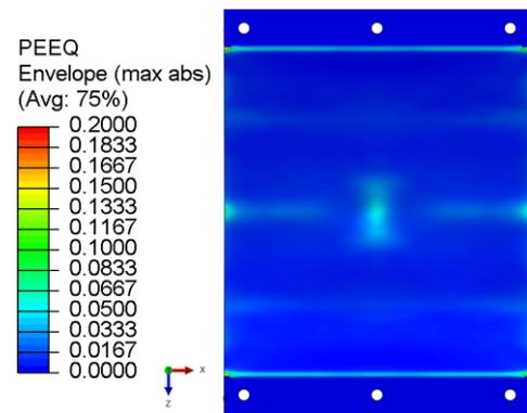
Fig 9. PEEQ accumulated on the sheet over the course of the simulation.
