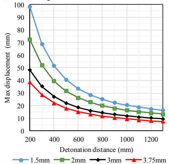
Fig 4. Max displacement at the sheet center as a function of detonation stand-off distance and steel sheet thickness
