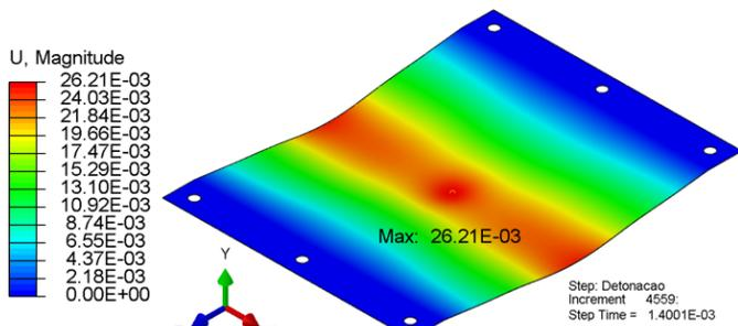
Fig 6. Displacement across example sheet at 1.4 ms.
