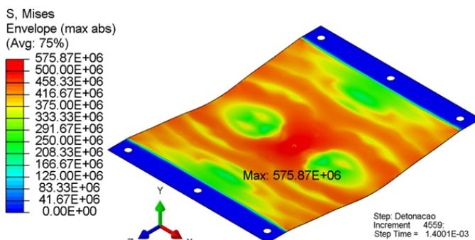
Fig 8. Von Mises Stress across example sheet at 1.4 ms.
