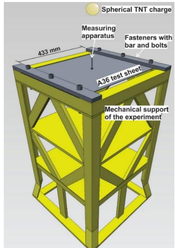
Fig. 1. Tests layout
