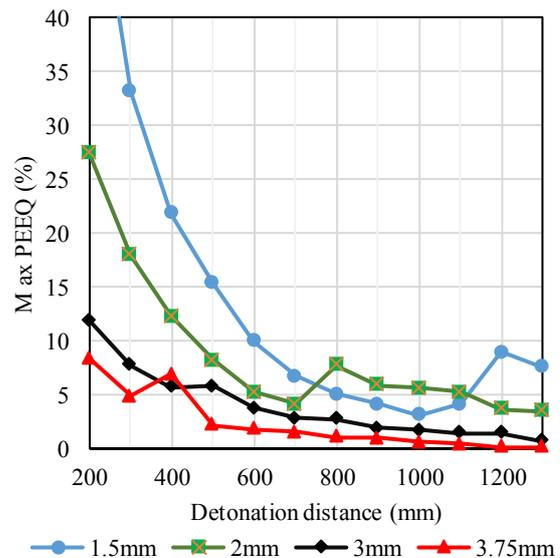
Fig 5. Max PEEQ at the sheet center as a function of detonation stand-off distance and steel sheet thickness
