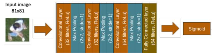
Fig. 2: CNN architecture from [8].
