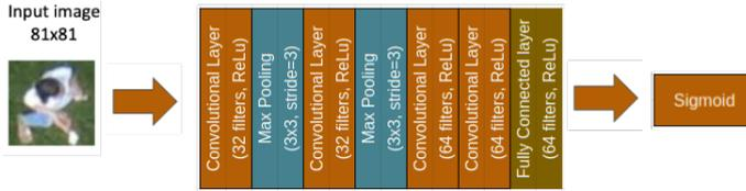
Fig. 3: CNN architecture from [4].
