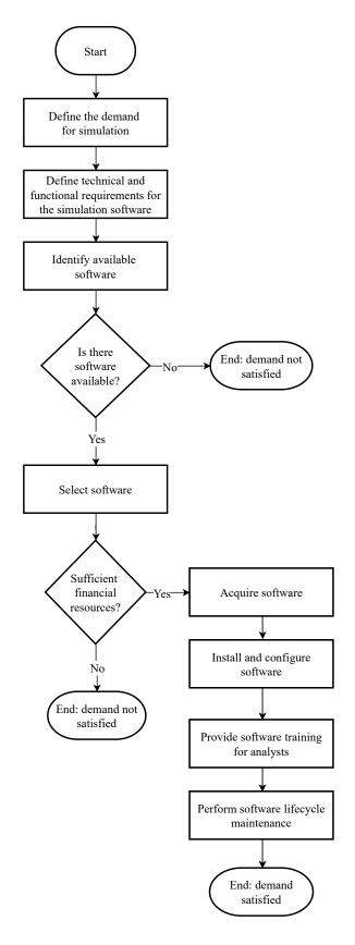
Fig. 2: Acquiring Simulation Software: A Typical Process Overview.
