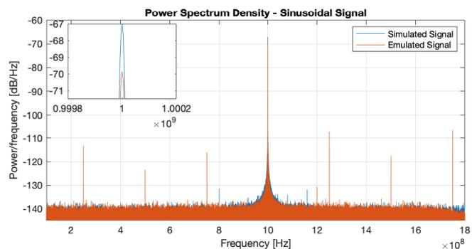
Fig. 9. Power spectral density of the sinusoidal pulse.
