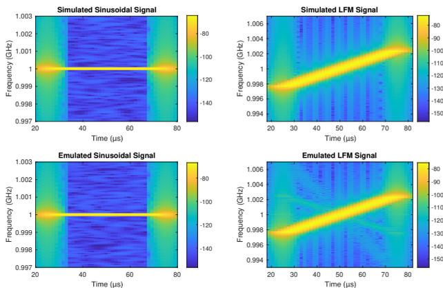
Fig. 11. Spectrogram of simulated and emulated pulses.
