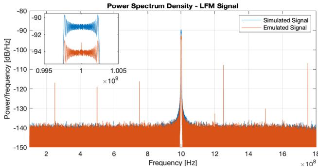
Fig. 10. Power spectral density of the LFM pulse.
