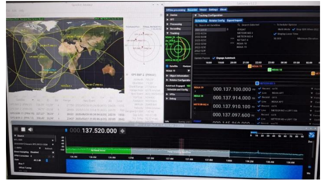
Fig. 2. Interface view combining GPredict (satellite tracking map) and SatDump (automated decoding and spectral visualization) during real-time reception in 137.5 MHz.
