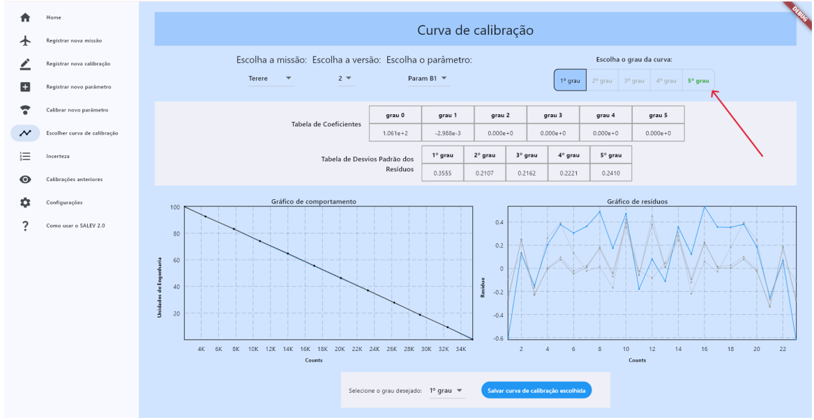
Fig. 1. SALEV 2.0 calibration page: polynomial fits, residual plot and coefficient/standard-deviation tables, with the F-test-recommended degree highlighted.
