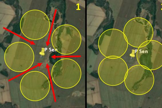
Fig. 1. Representation of the theoretical coverage of a radar network.
